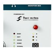
If at any time the status LED turns off during normal operation please check all connections and if further problems develop please contact Audient support.
