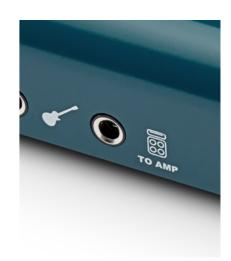
To send audio to the To Amp output, simply send the audio to Output 3 (To Amp) in your DAW and connect a jack to the To Amp output.
