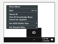
Once installed, the iD mixer can be opened by going to the system tray and right clicking the iD icon. Right-click to quit or change buffer and sample rate settings.
