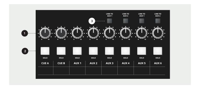
The auxiliary masters control the overall level of the auxiliary outputs. A balance or mix can thus be created by using the controls on the channel strips and the overall level adjusted by using the auxiliary master control. The auxiliary outputs can be solo'd so that a balance can be created by listening to the output.
