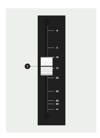
The master fader is used to control the stereo output of the console. Unlike the channel faders it is calibrated with the OdB mark at the top as the main purpose of this fader is to create a fade out at the end of a title.
