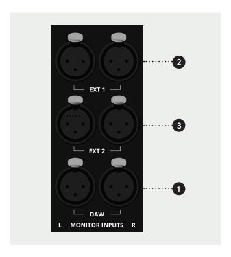
This panel carries the connectors for the external inputs to the monitoring system.
