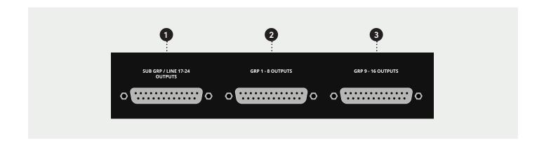
Rather than having individual connectors for each bus and sub-group output it is much more convenient (and quicker to make a connection) if they are on D-sub multi-pole connectors.
