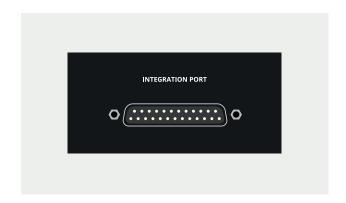
On the Rear of the Console, you will find the Integration Port allowing you to synchronize the console with an external monitor controller. This port provides a copy of the Control Room Output, a Stereo Guide track which is fed from AUX 5+6, as well as DC outputs to synchronize the SOLO and DIM status of the Console with an external Monitor Controller.
