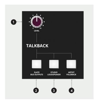
The Talkback Microphone input has 48v Phantom enabled by default so condenser mics can be used. This can be disabled by removing an internal link. Contact Audient support for more information.
