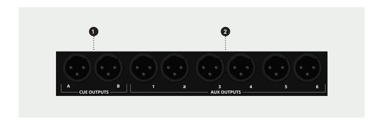
The auxiliary outputs are typically used to send to effect units such as reverberation units. They are line level fully balanced outputs.
