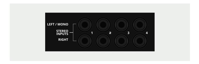
This panel carries the input TRS jacks for the stereo inputs located on the master section of the console.
