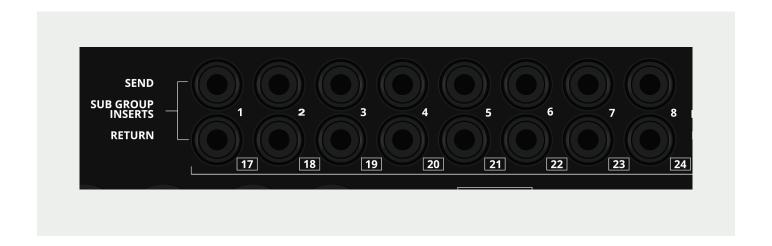
This panel carries the connectors for the sub-group insert points. There are 8 sub-groups and each insert point has a send output and a return input.
