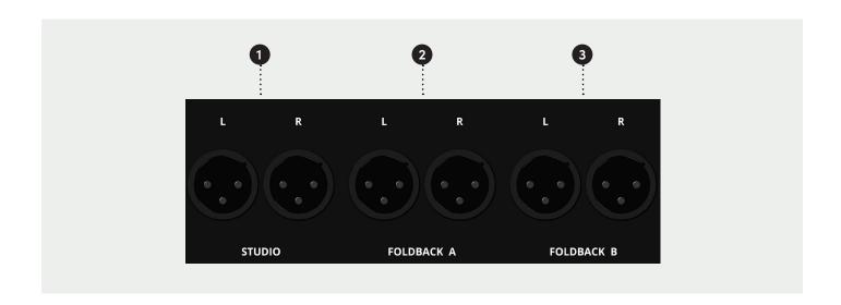
These are the XLR connectors for the Studio Loudspeaker and the two foldback outputs. Each output is stereo, having a left and right connector.
