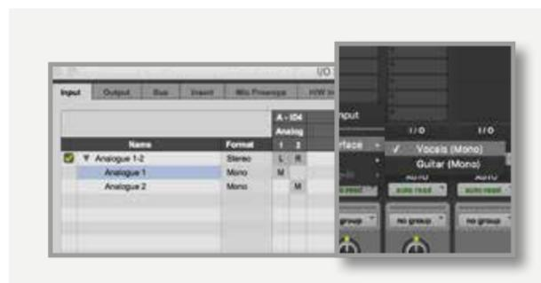
If using the iD4 Monitor Mix knob to monitor your inputs, ensure that the input monitor buttons on the audio tracks are not selected, to avoid duplicate signals.
