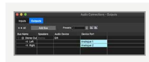
If using the iD4 Monitor Mix knob to monitor your inputs, ensure that input monitoring is turned off on the track.
