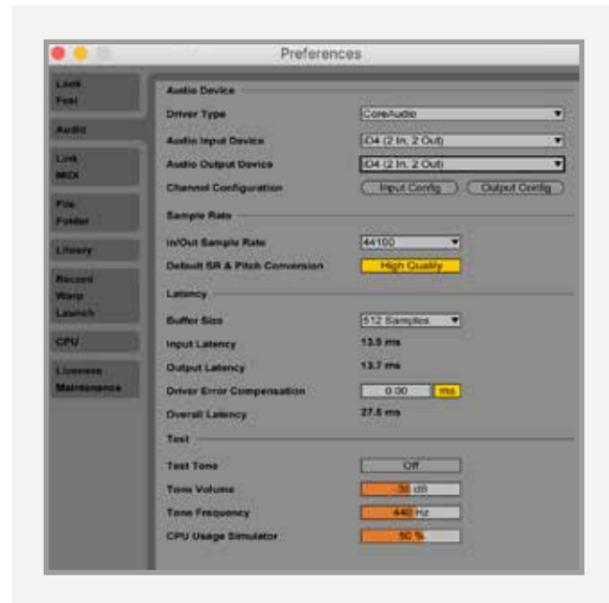
If you are monitoring your inputs using the Monitor Mix knob, then you can keep the buffer size reasonably high to reduce the strain on your computer. In this case, you also need to make sure that input monitoring is turned off on the track in Ableton.
